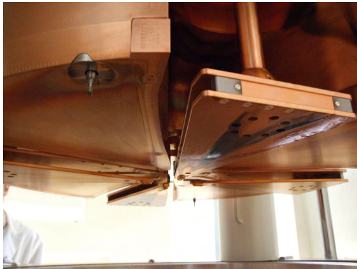
Pie shaped wedges are the Dees, which accelerate the protons. Just left of the Dee is the specially shaped trim bar. Silver part is where the extractor foil carousel will be mounted.
