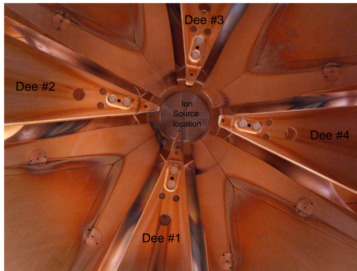
View looking up at the Dees and hills. Steel plug in the center is where the ion source will drop in. Note the Dees have different lengths based on position.
