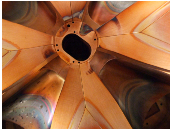
View looking down where hills meet together. Central hole is for the base of the ion source. One diffusion pump is located directly under the ion source.
