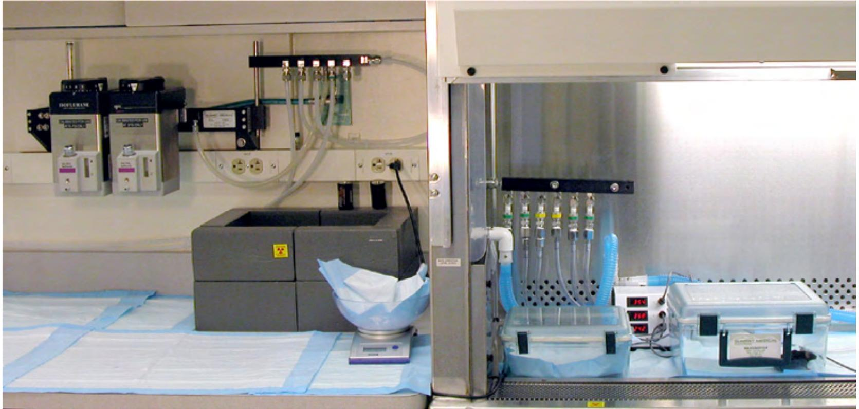
Wall mounted gas anesthesia provides easy to use constant depth of anesthesia. Variable anesthesia can lead to movement, physiological changes altering blood flow, clearance and probe delivery.
