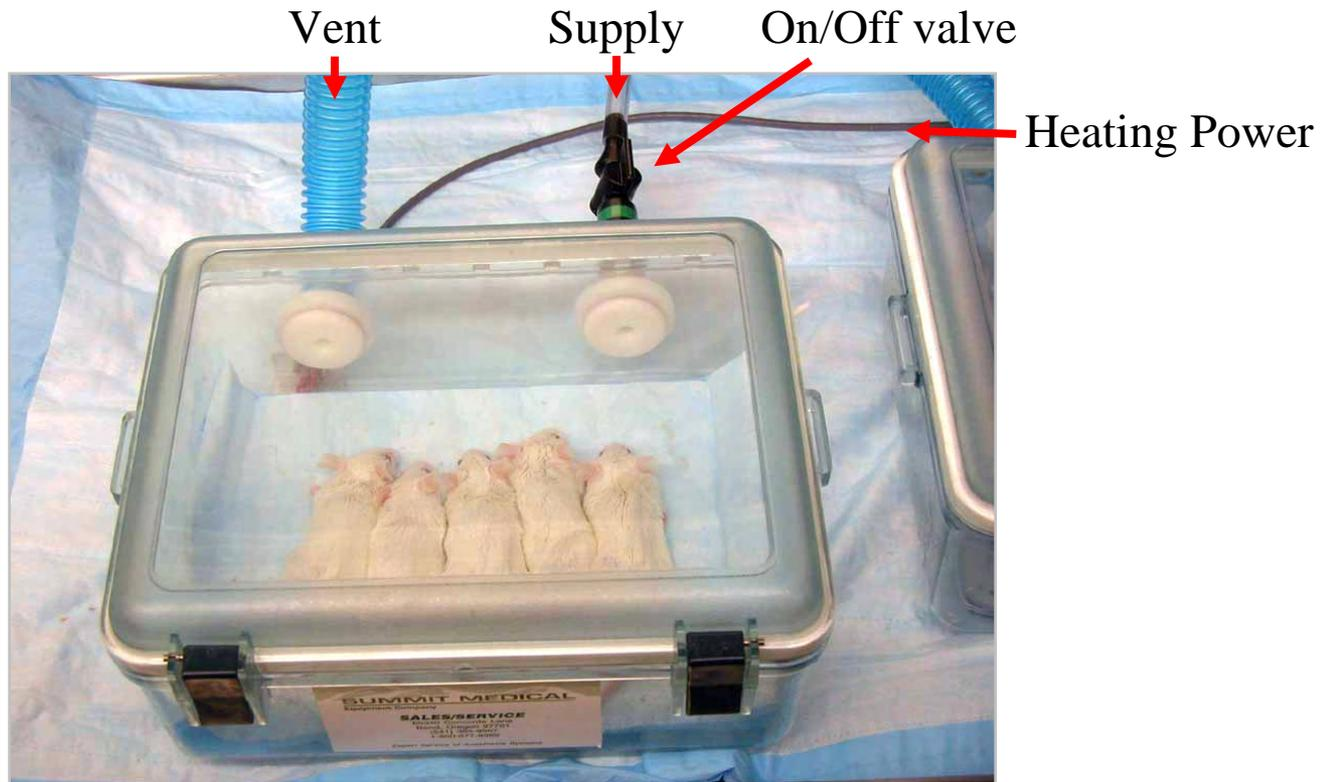
A fast, simple, easy to use box that can be used for multiple animals. Anesthesia is delivered and removed via ports at the rear of the box. Animals are kept warm by a heating plate located under the box. Easily sterilized using spray bottle containing Virkane or Trifectant.
