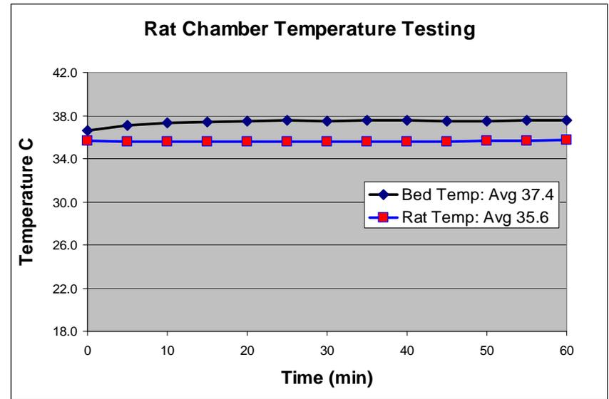
Mice and rats both quickly equilibrate to the sled temperature when under anesthesia. Regulated feedback control is essential to ensure that rodents are not overheated. Physiological tolerance for overheating is much less than colder conditions.
